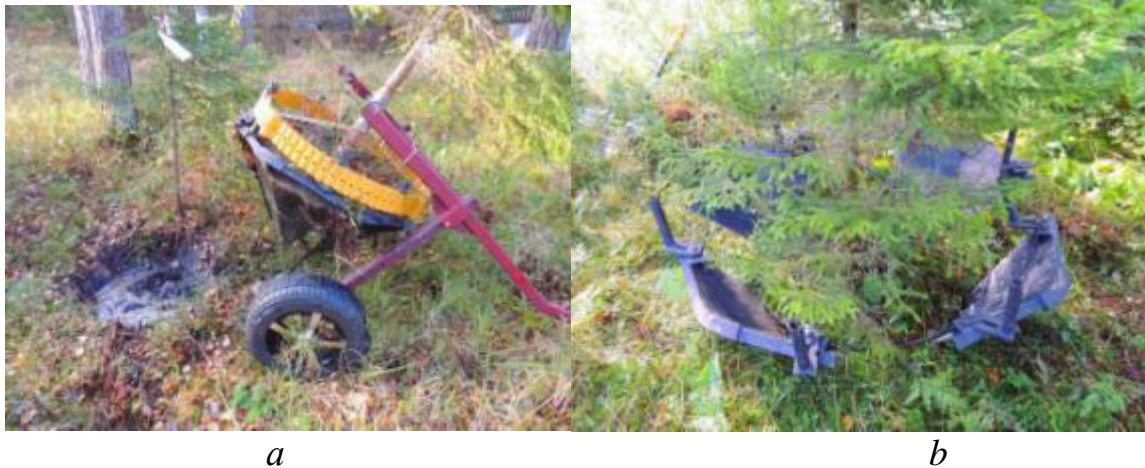
Picture 1 - The device with manual sinking for transplanting seedlings: a-installation of bucket-shaped knives in the specified order; b-extraction of the seedling from the ground
