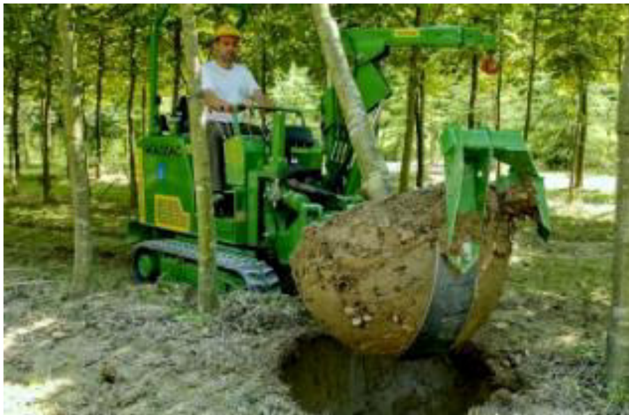
Picture 5 - The mechanism for transplanting seedlings with a rotary vibrating knife
