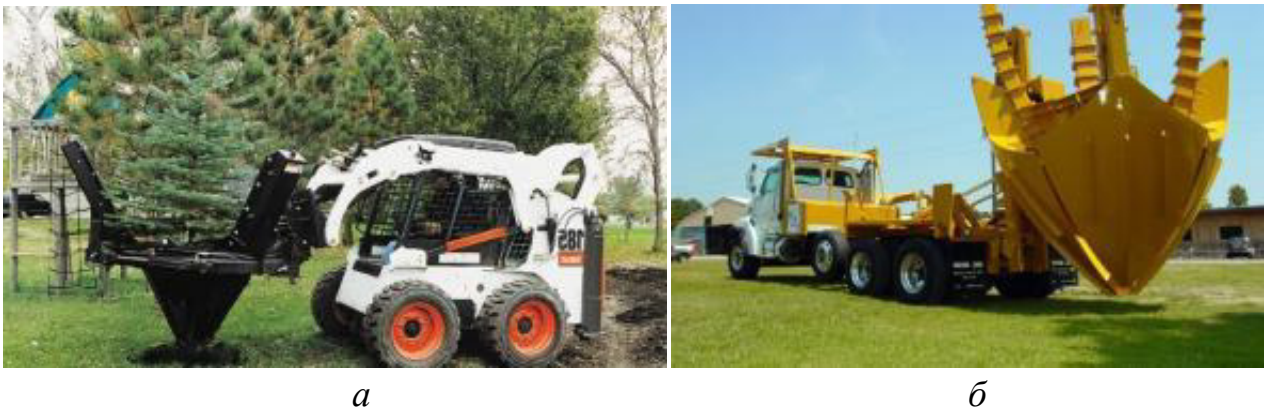
Picture 3 - Application of bucket knife design in units with various mobile power tools: a-compact version for transplanting seedlings; b - large-sized version for transplanting trees
